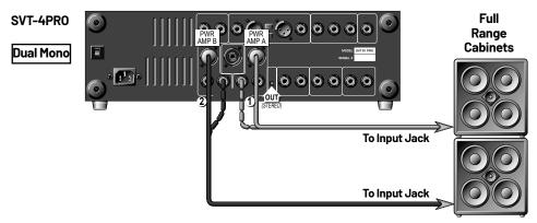
In the above **Dual Mono** example, each of the SVT-4PRO internal power amplifiers will power a set of full range cabinets. Disengage the Stereo/Mono Bridge switch (Stereo position). Connect a speaker cable from the SVT-4PRO - Power Amp A Speaker Output jack to the input jack(s) of a set of full range speakers. Next, connect a speaker cable from the SVT-4PRO - Power Amp B Speaker Output jack to the input jack(s) of another set of full range speakers.
