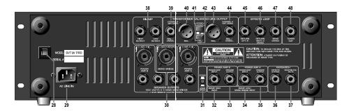
28. CIRCUIT BREAKER: The SVT-4PRO employs an AC line Circuit Breaker to help protect against damages due to excessive current demands. If the amplifier stops working, check this Circuit Breaker.
