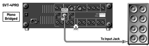
In the above **Mono Bridged** example, both the SVT-4PRO internal power amplifiers are bridged together to produce maximum output power. Engage the Stereo/Mono Bridge switch (Mono Bridge position). Connect a heavy duty speaker cable terminated with a speakON connector (pin 1+ = positive, pin 1- = negative) from the SVT-4PRO Mono Bridge Output jack to the input jack of a speaker cabinet capable of handling the extremely high output power.
